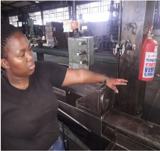
Zama with the hand safety device that she designed and built for the draw benches.
